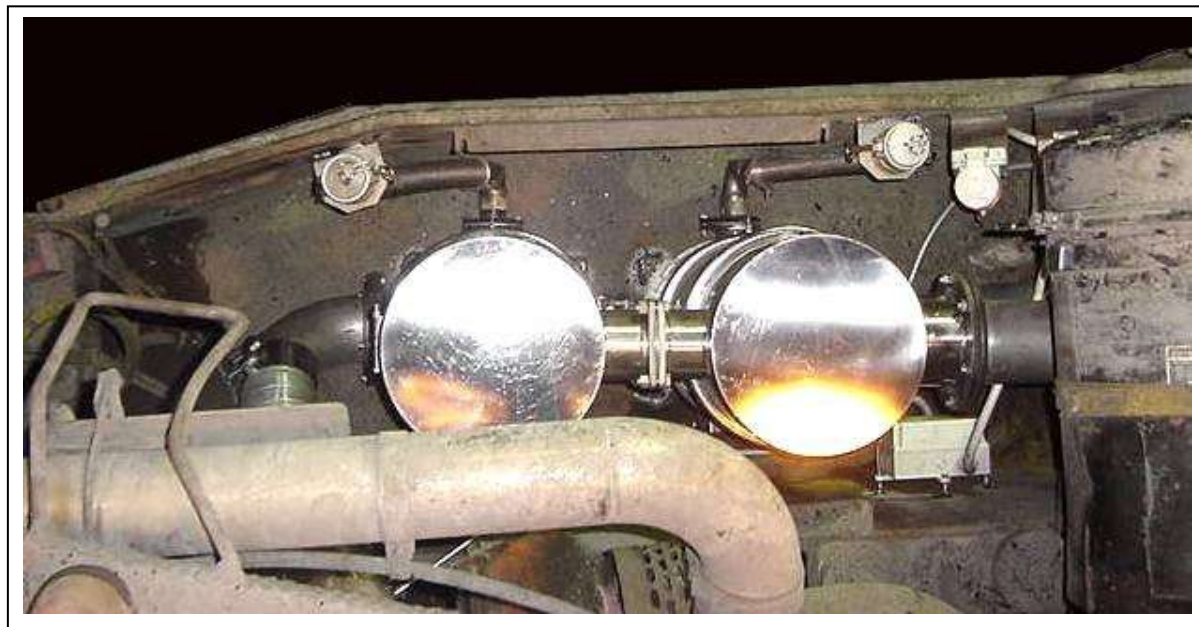
Figure 43: Top view of installed ECS Combifilters
