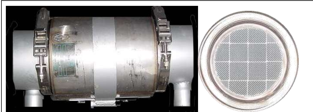
Figure 38: DCL Titan DPF, side view on the left and end view on the right. The side view shows the two end caps connected to the main canister by quick disconnect clamps.
