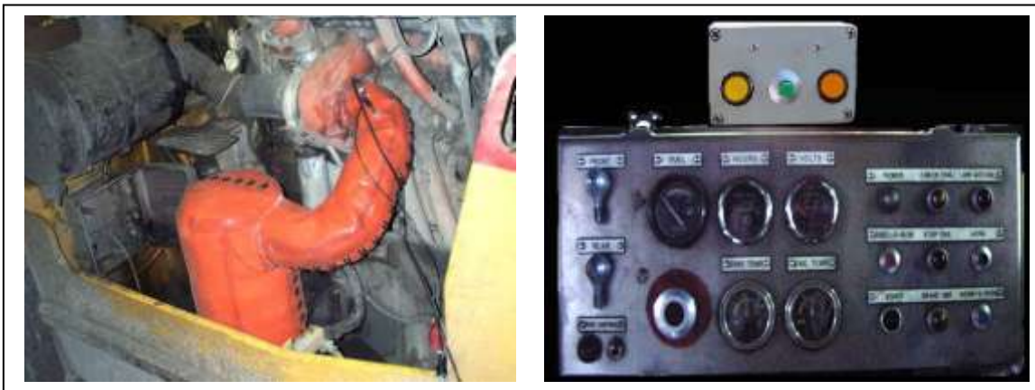
Figure 37: Engelhard DPX2 DPF as installed with insulation (left) and backpressure monitor on dash (right).
