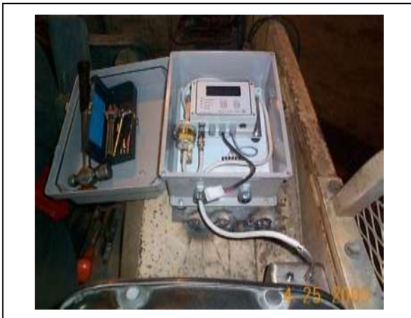
Figure 19: Installation of data logger just behind driver's seat on a Kubota tractor
