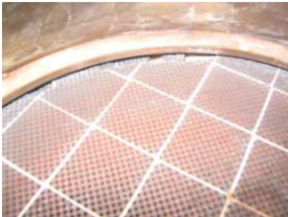
Figure 135: Separation of SiC filter from canister ring (top of photo).
