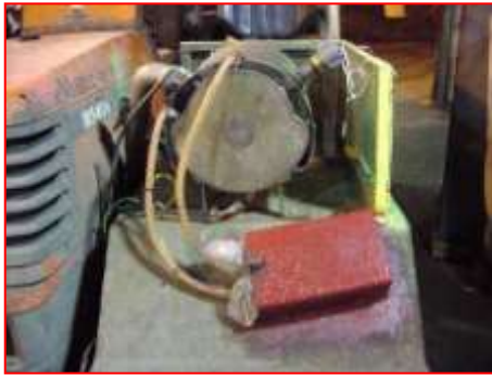
Figure 32: ECS/3M Omega filter mounted on tractor #2180. The yellow cage was to prevent operator contact with hot surfaces. The red box on the fender is a protective casing containing the power connector for electrical regeneration.
