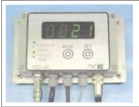
Figure 15: As-received data logger. The five I/O ports (left to right) are for pressure, two temperature sensors, engine rpm, power, and alarm outputs.
