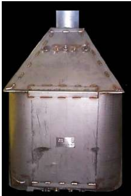
Figure 24: O-M housing containing eight filter cartridges.
