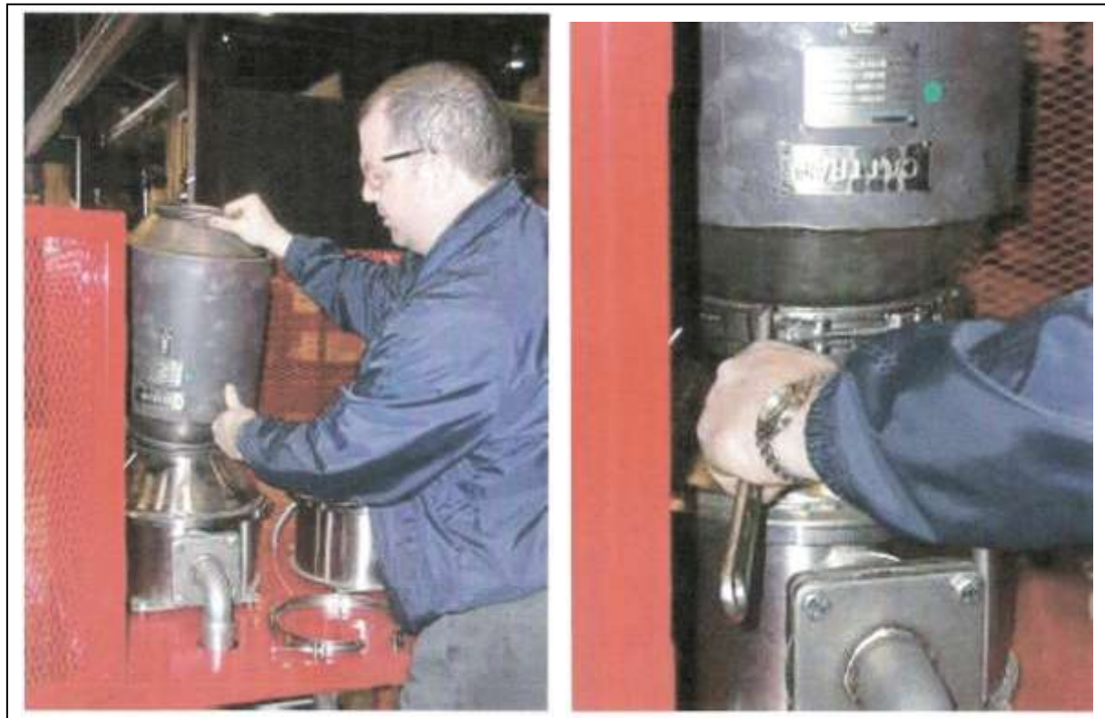
Figure 49: Mounting a loaded DPF on the CombiClean heater (left) and securing it with gasket and clamp (right).
