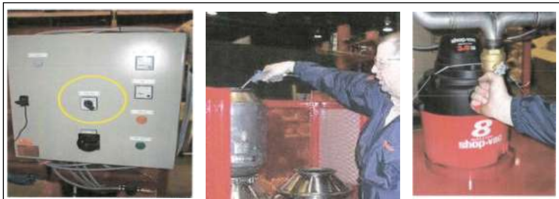
Figure 50: The CombiClean control panel (left), access for sweeping compressed air across the outlet side of the DPF filter element (middle) and vacuum system valve (right).
