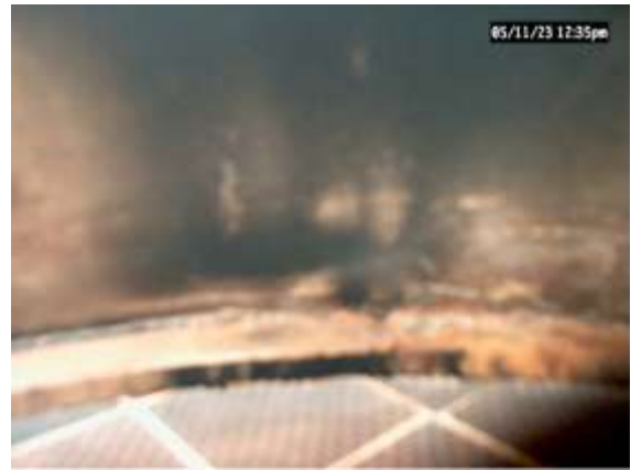
Figure 136: Blackened soot shadow at points of monolith separation indicating unfiltered exhaust bypassing filter.
