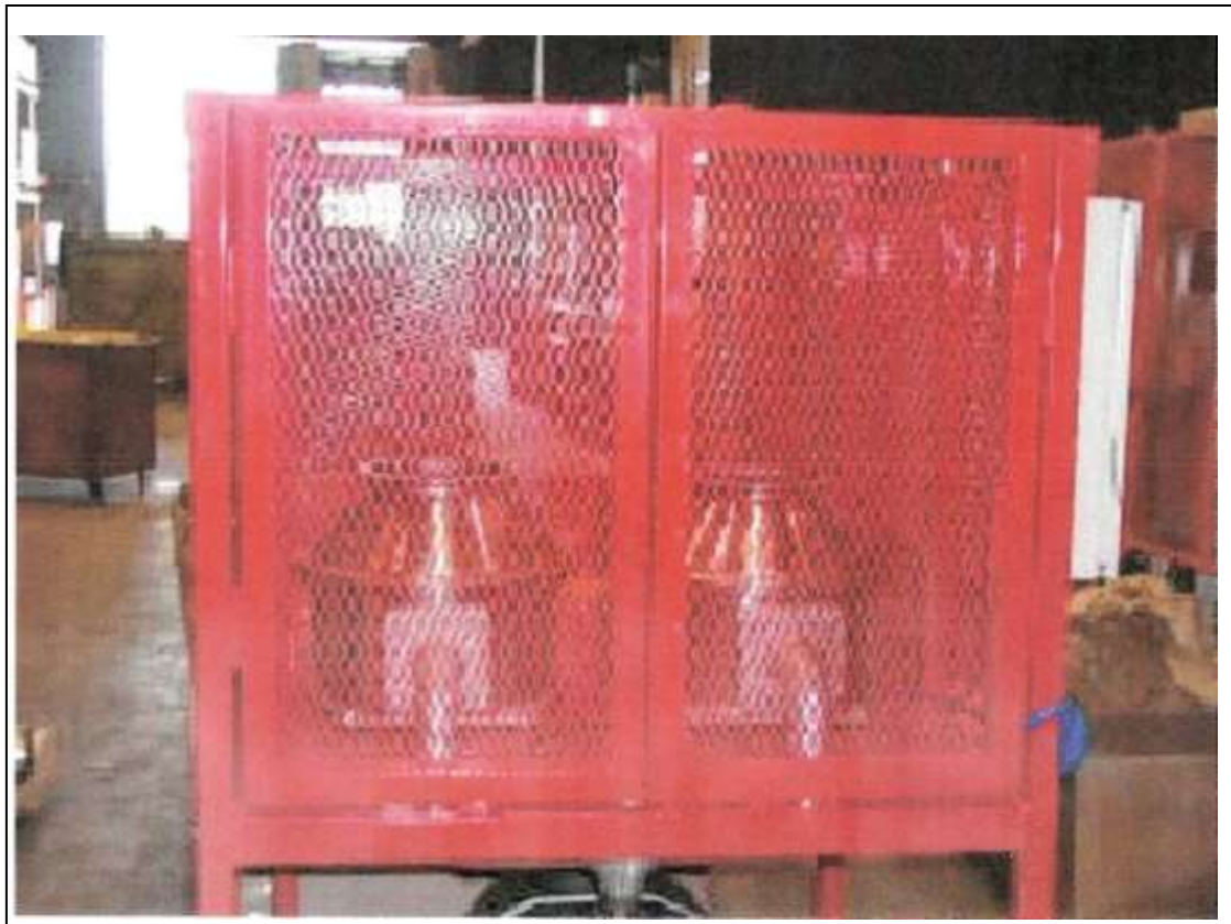
Figure 48: The ECS CombiClean™ DPF regeneration system, consisting of two heating compartments. Below what is shown is a shop type vacuum system (see Figure 50) used in conjunction with compressed air jet at the beginning of the regeneration process to remove the bulk of soot and ash.
