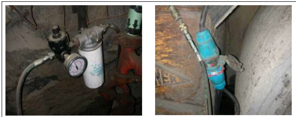
Figure 31: Air line with moisture removal and pressure gauge (left). The electrical connector (blue) and air line to its left (right).
