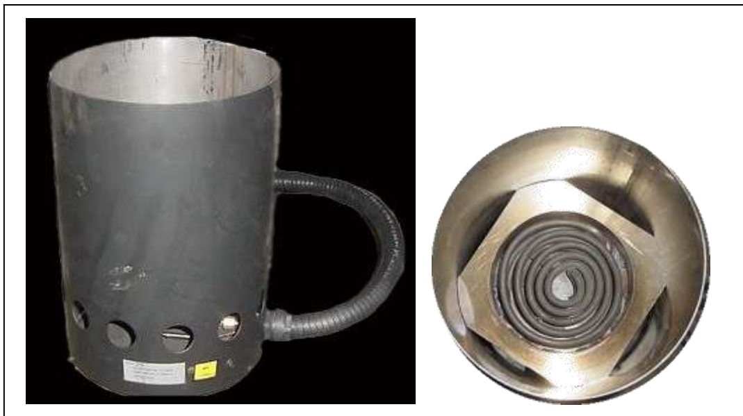
Figure 41: Regeneration "cooker" for DCL Titan DPFs: side view (left) and top view showing heater elements (right).
