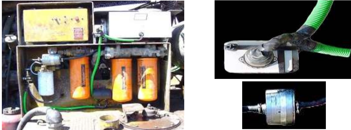
Figure 25: O-M FBC dosing components. Left: overall system; Upper right: electronic dosing control; Lower right: dosing pump.
