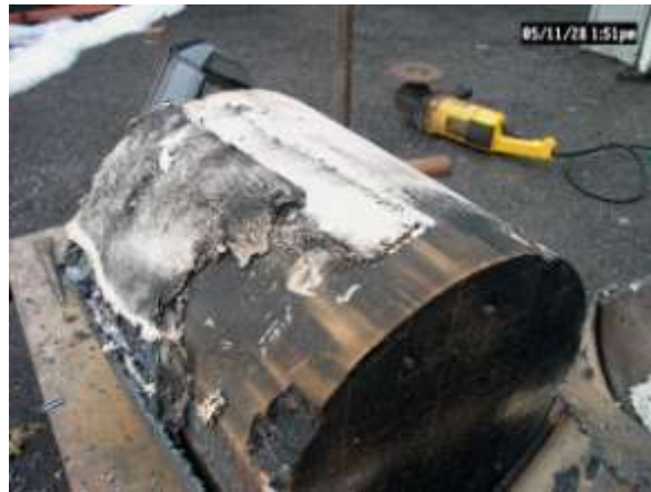
Figure 134: Degradation of mat holding J-M filter element in place.
