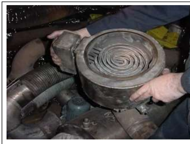
Figure 27: Heating element at the bottom of the JM DPF system.
