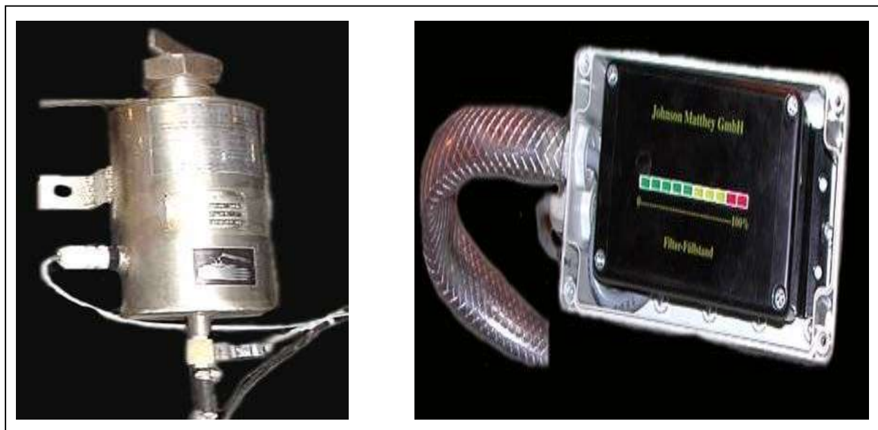
Figure 29: Automatic FBC dosing equipment (left) and backpressure monitoring display on dash (right).
