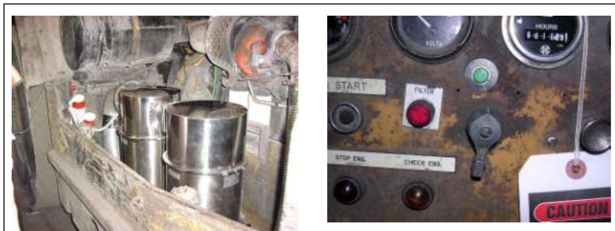
Figure 44: Side view of Combifilters (left) and backpressure monitor on dash (right).
