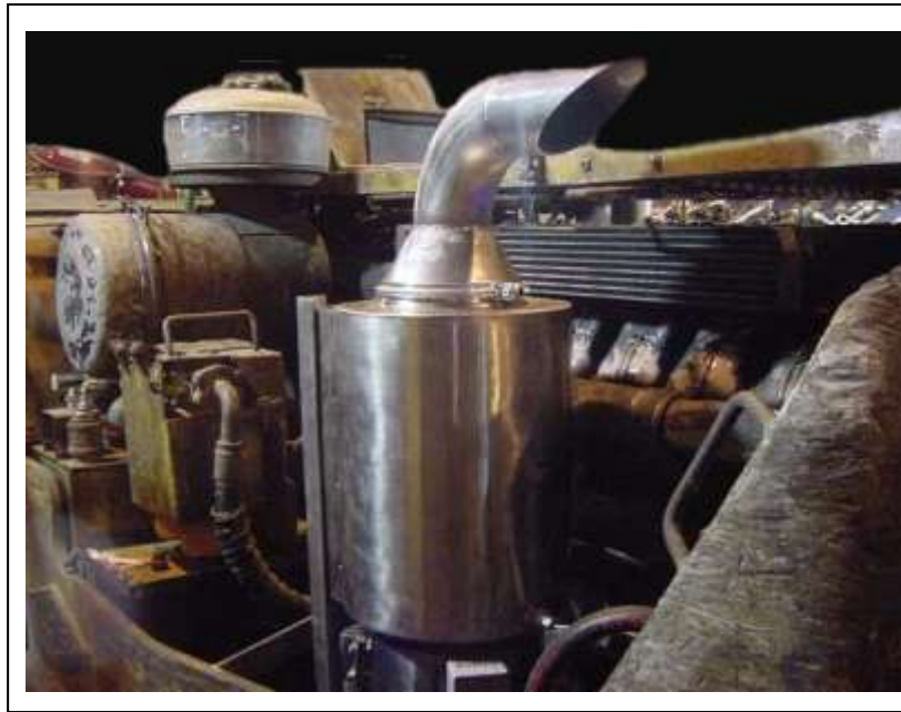
Figure 28: One of two JM filters mounted on either side of the dual exhaust Deutz V-12 engine.
