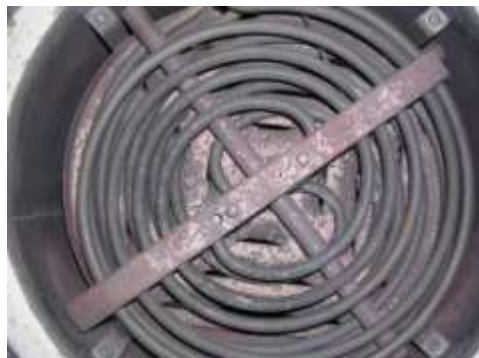
Figure 126: Inside of oven after seven “cookings” of the ECS DPF.
