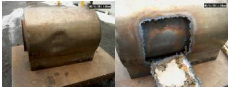
Figure 133: Johnson Matthey outer shell dent (right) and undamaged inner canister (left).
