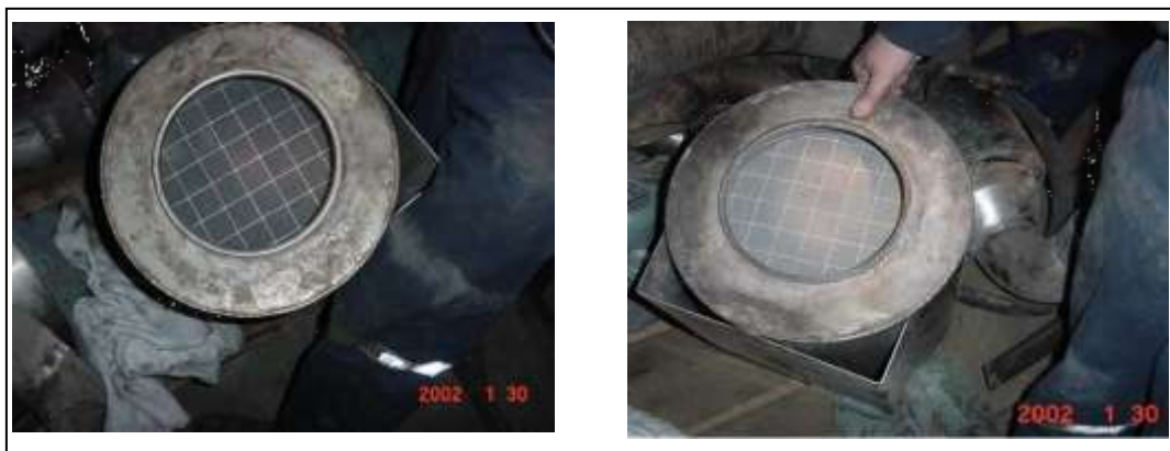
Figure 105: The inlet side (left) and discharge side (right) of the Johnson Matthey DPF on left of LHD #820.
