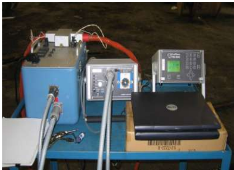
Figure 55: PAS 2000 photoelectric aerosol analyzer (on the right) with the dilution equipment on the left.
