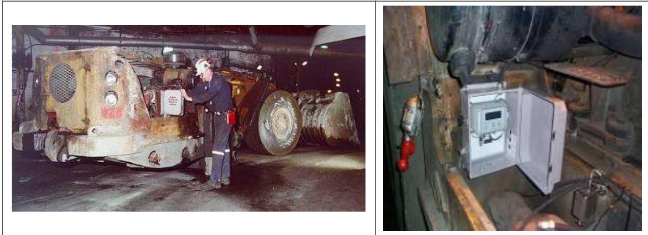
Figure 18: Installation of data loggers on LHDs.
