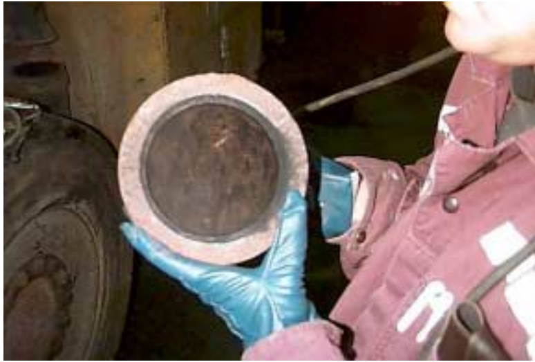
Figure 4 - Using a Light To Check For Carbon Buildup
