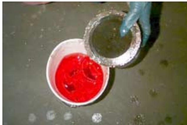
Figure 3 - Cleaning Oxy Catalyst in Fuel
