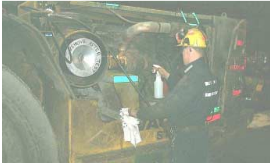
Figure 2 - Checking Intake For Leaks
