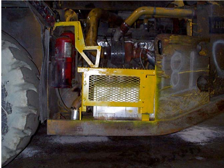
Figure 19 - Original Oberland Mangold DPF Installation
