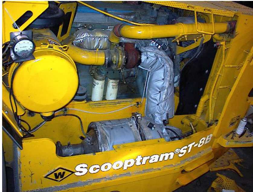
Figure 15 - DCL Bluesky Installation on VL247
