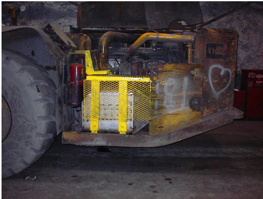
Figure 20 - Final Oberland Mangold DPF Installation
