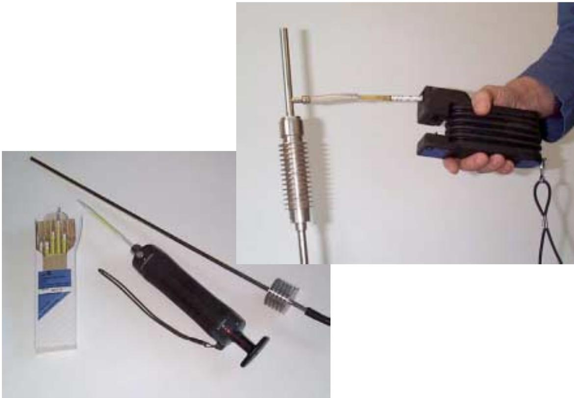
Figure 7. Carbon monoxide sampling using gas tubes
