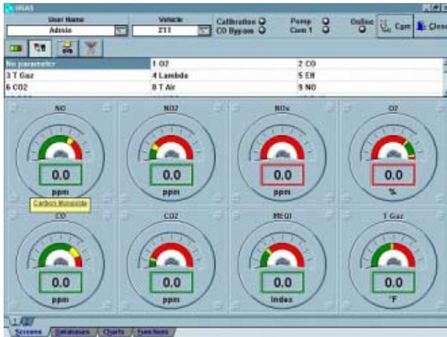
Figure 6. UGAS software control panel
