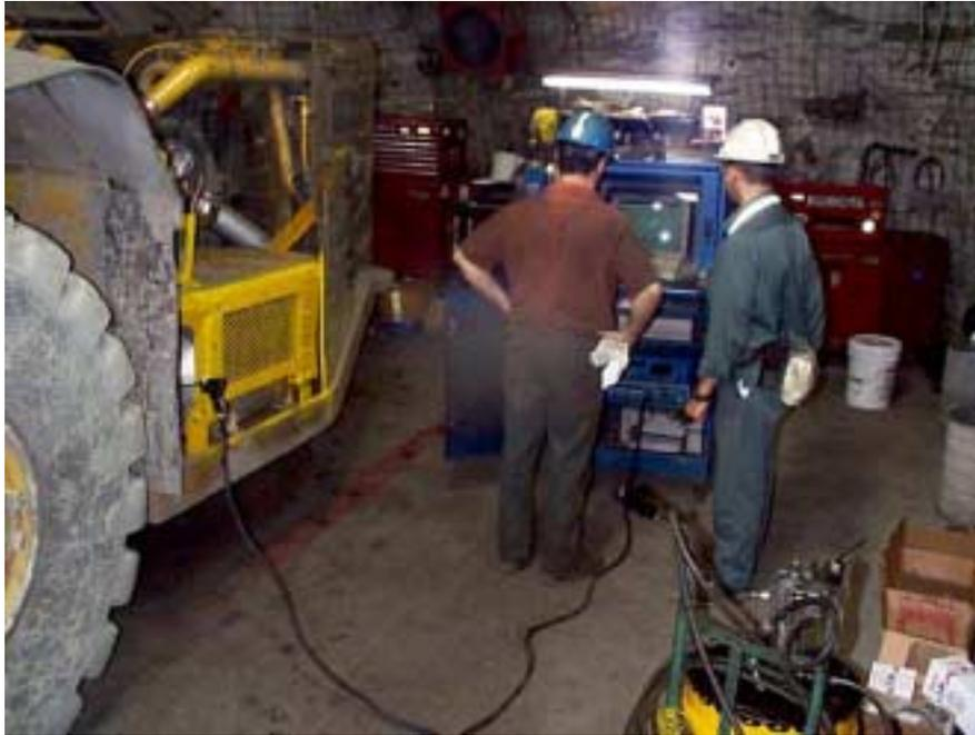
Figure 5. UGAS/ECOM direct exhaust sampling
