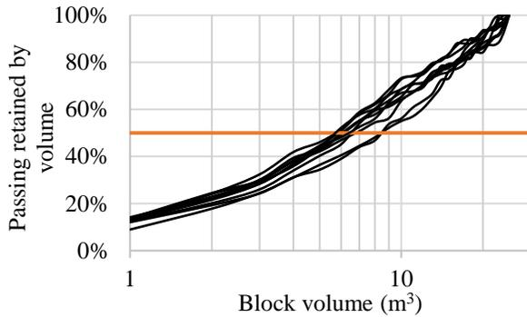
Figure 9. IBSD estimations for all ten DFN realizations. 50% passing line shown in orange.
