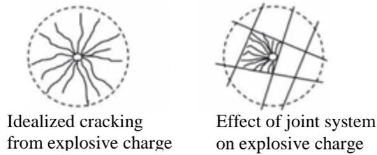
Figure 1. The effects of a joint system on fragmentation (after Singh *et al.*, 2016).
