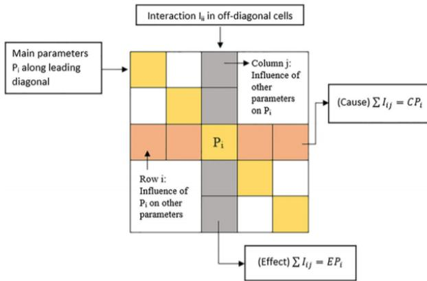
Figure 4. A generalized view of an RES interaction matrix (From Hasanipanah *et al.* 2016)
