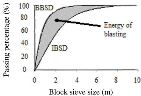
Figure 3. The comminution concept applied to blasting: the IBSD is converted to the BBSD by explosive energy (after Latham *et al.*, 1999)
