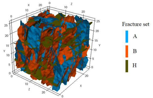
Figure 5. Single realization of the DFN model (250 fractures) used to quantify fracture network parameters for inclusion in an RES solution for a blast fragmentation index.
