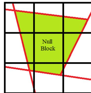
Figure 8. A null block is the smallest possible estimation of an *in situ* block (green). Fracture traces are shown in red for a 2 dimensional representation.
