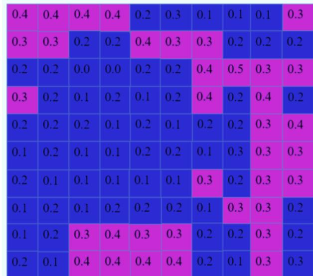
Figure 11. P<sub>32</sub> fracture intensity shown as a heat map for DFN realization #5 (a) and #6 (b). Colors are coded as shown in legend.
