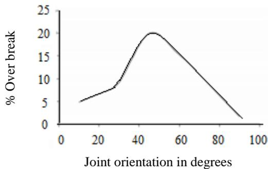
Figure 2. Observed over break in relation to the orientation of fracture sets with respect to the free face (after Singh, 2006).
