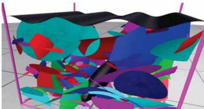
Discrete fracture network with excavation boundaries
